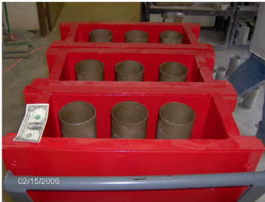
Figure 3-9. Experimental Slab Forms.
