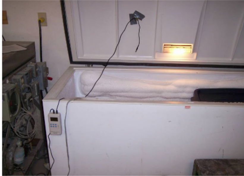
Figure 3-7: Chamber for 33 F Curing (Outside)
