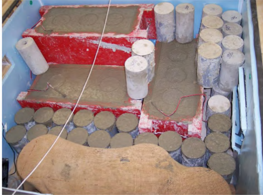
Figure 3-2: Inside a Curing Chamber
