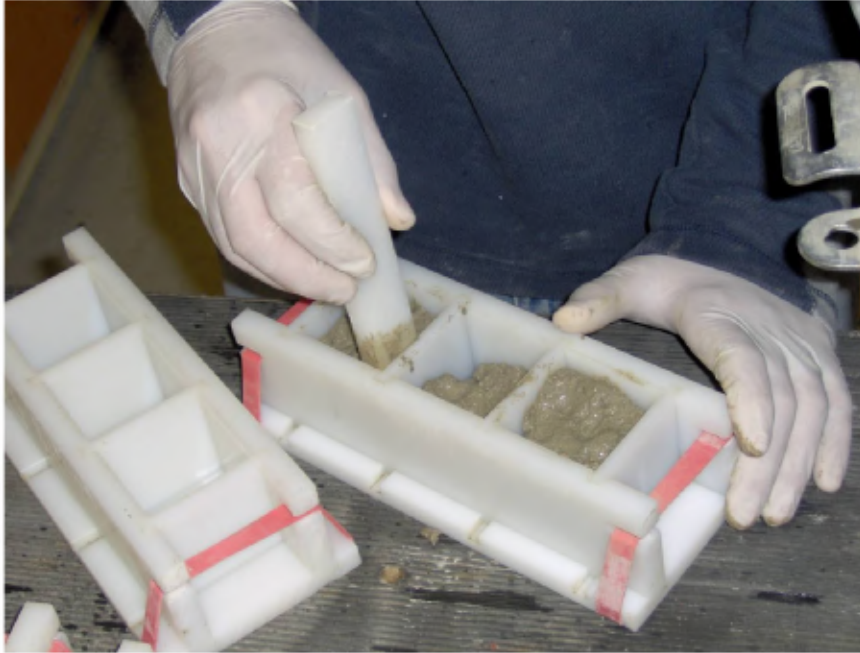
Figure 3-13. Mortar Cube Casting.
