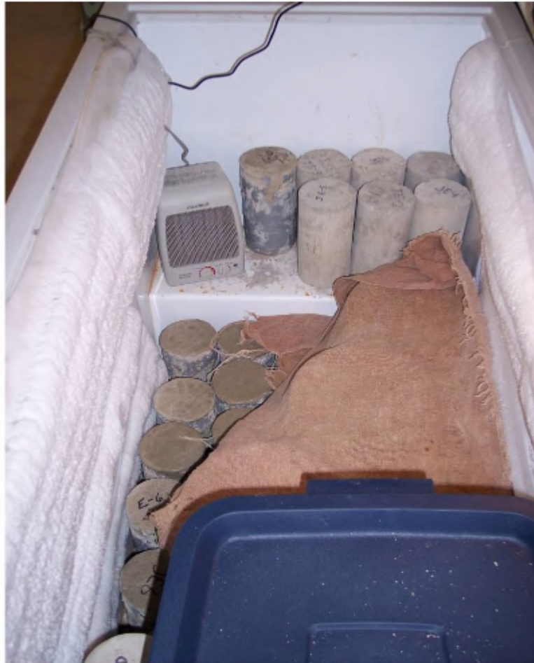
Figure 3-6: Chamber for 33 F Curing (Inside)
