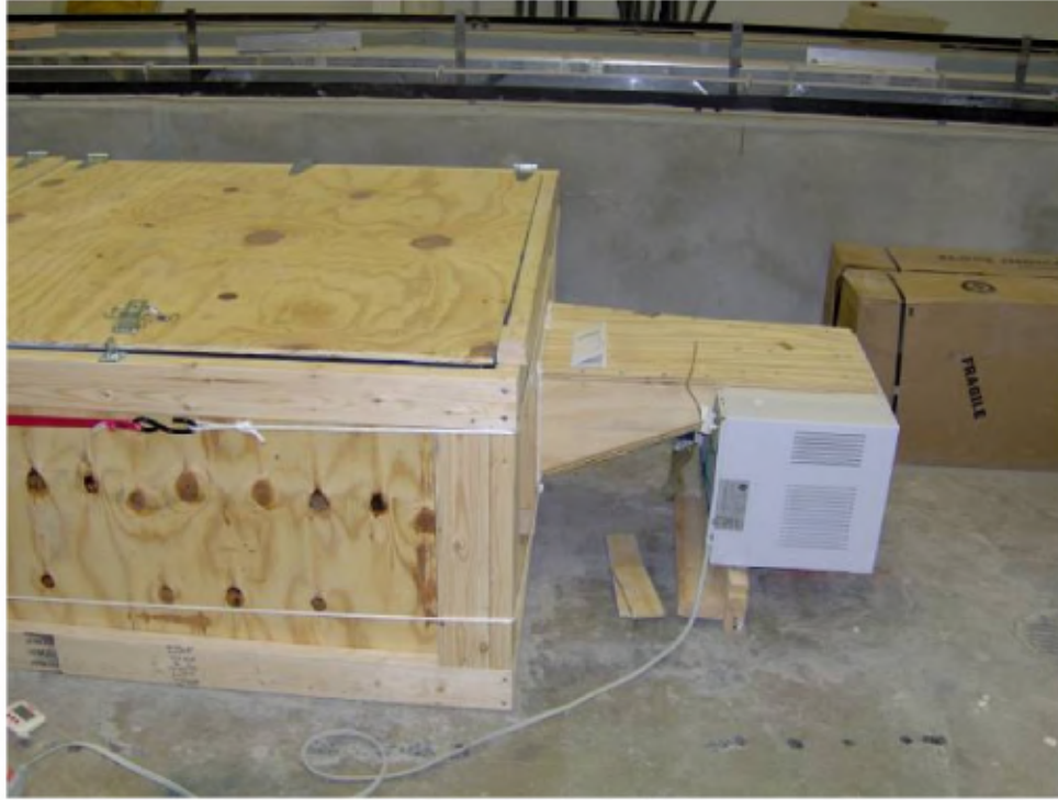
Figure 3-1: The Curing Chambers (before insulating the A/C unit)
