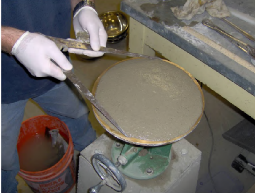
Figure 3-12. Flow Test Measurement.
